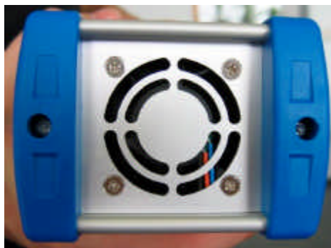
Air exhaust with fan
