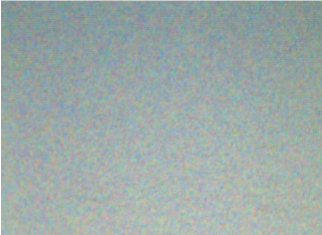
White light illumination: Sparkle is obvious as random modulations of intensity and chromaticity.
