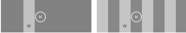
Line of width w , fixed measurement field M Array of lines of width w (grille, grating)
