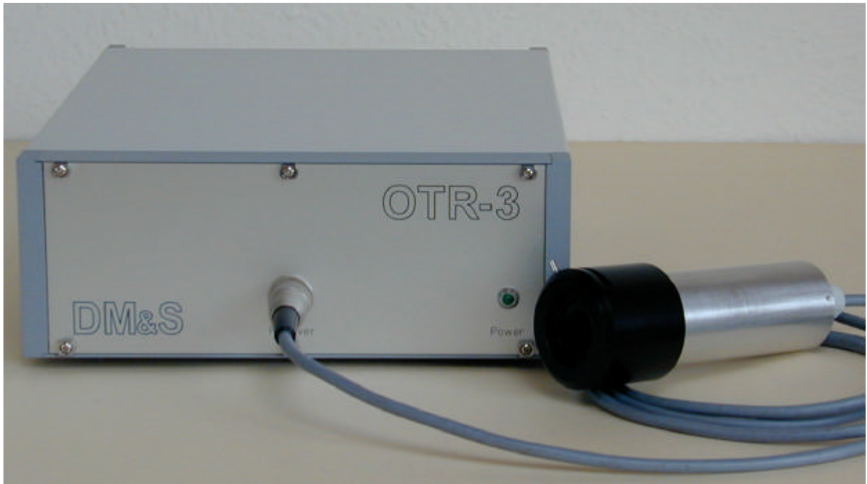
OTR-3 electronics box and collimating receiver, measurement field diameter continuously adjustable from 25 mm to zero (for measurement of dark-signal).
