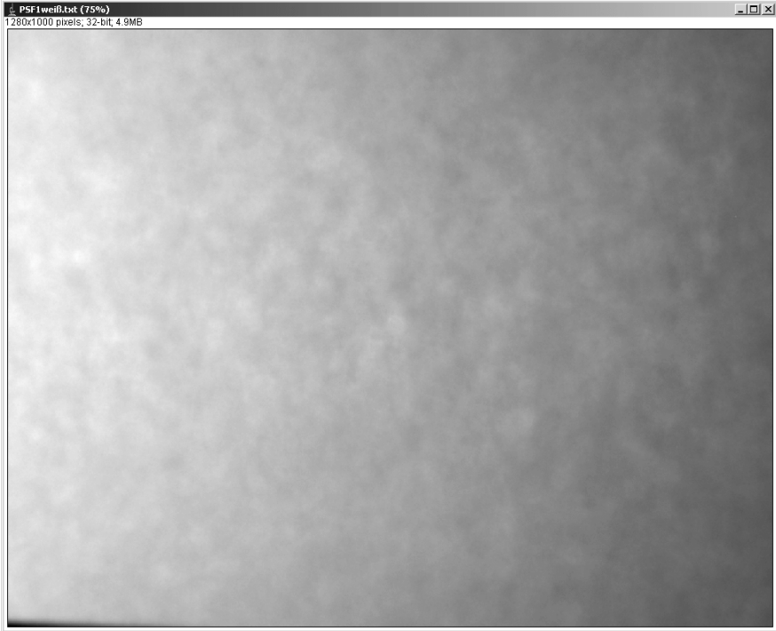
PSF lateral luminance distribution of the reflectance reference measured with an imaging photometer.
