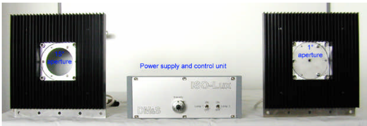
Figure 3: Components of the ISO-Lux illumination system: light-source with 15^\circ aperture (left), stabilized adjustable current-source (center) and light-source with additional 1^\circ aperture attached (right).
