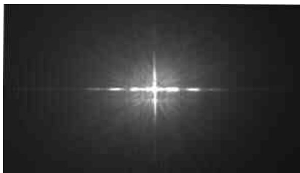
Figure 1: Luminance distribution obtained by reflection of a point-source in an LCD-monitor (point-spread-function, PSF).
